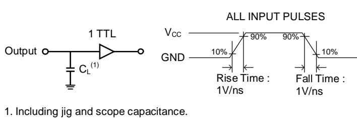
1. Including jig and scope capacitance.
